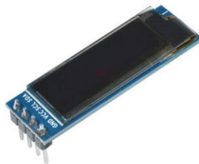
Figura 31. Display OLED 0.91" 128×32 I2C.
