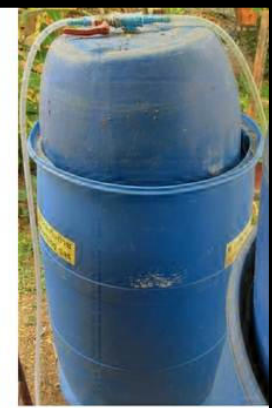
Figure 2. Bioreactor with some biogas
