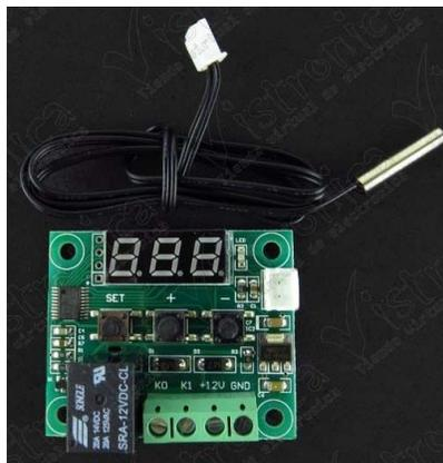
Figura 2. Termostato digital xh-w1209 [55].
